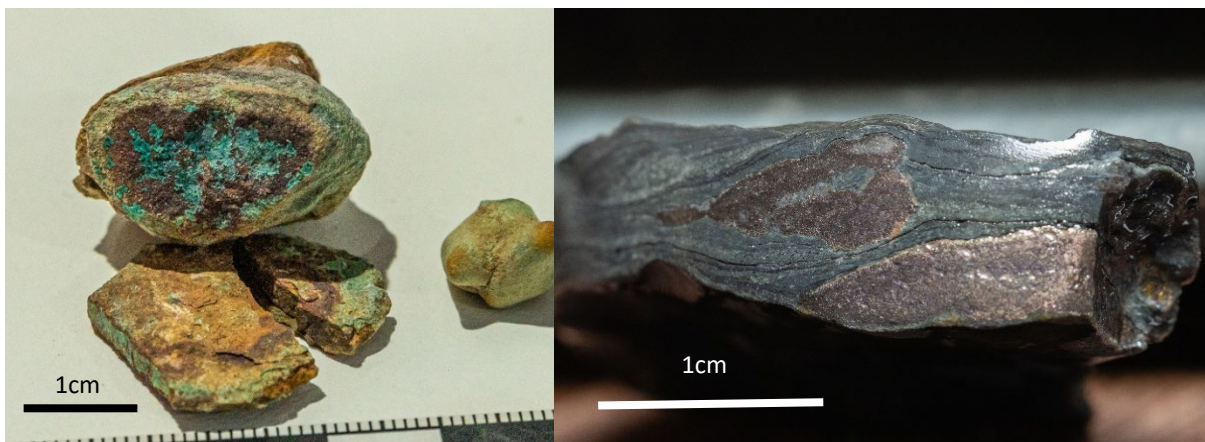
Photo 1 (left) – weathered copper rich nodules collected from surface at Area 1 (refer Figure 1) - containing malachite (interpreted after bornite-chalcopyrite), visual estimate 10% malachite in 2.5cm diameter nodule
