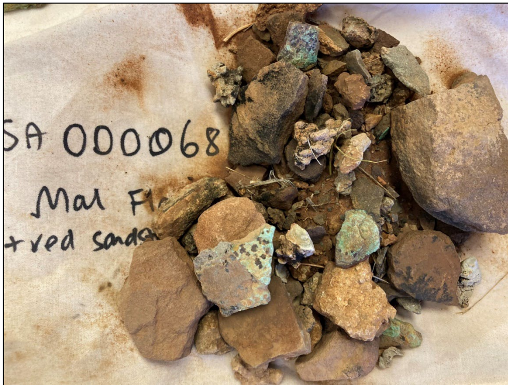
Photo 3 – Sample SA0000068 of surface scree containing malachite (Area 5)
